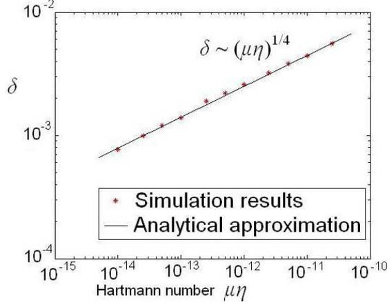
**FIGURE 2.** The thickness of the boundary layer from simulations is plotted as a function of the Hartmann number. The Analytical approximation fits with simulation results.
