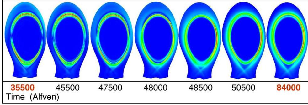
**FIGURE 5.** Transition between a predominantly  $m = 1$  flow to an  $m = 0$  flow structure with an increase in the kinetic energy
