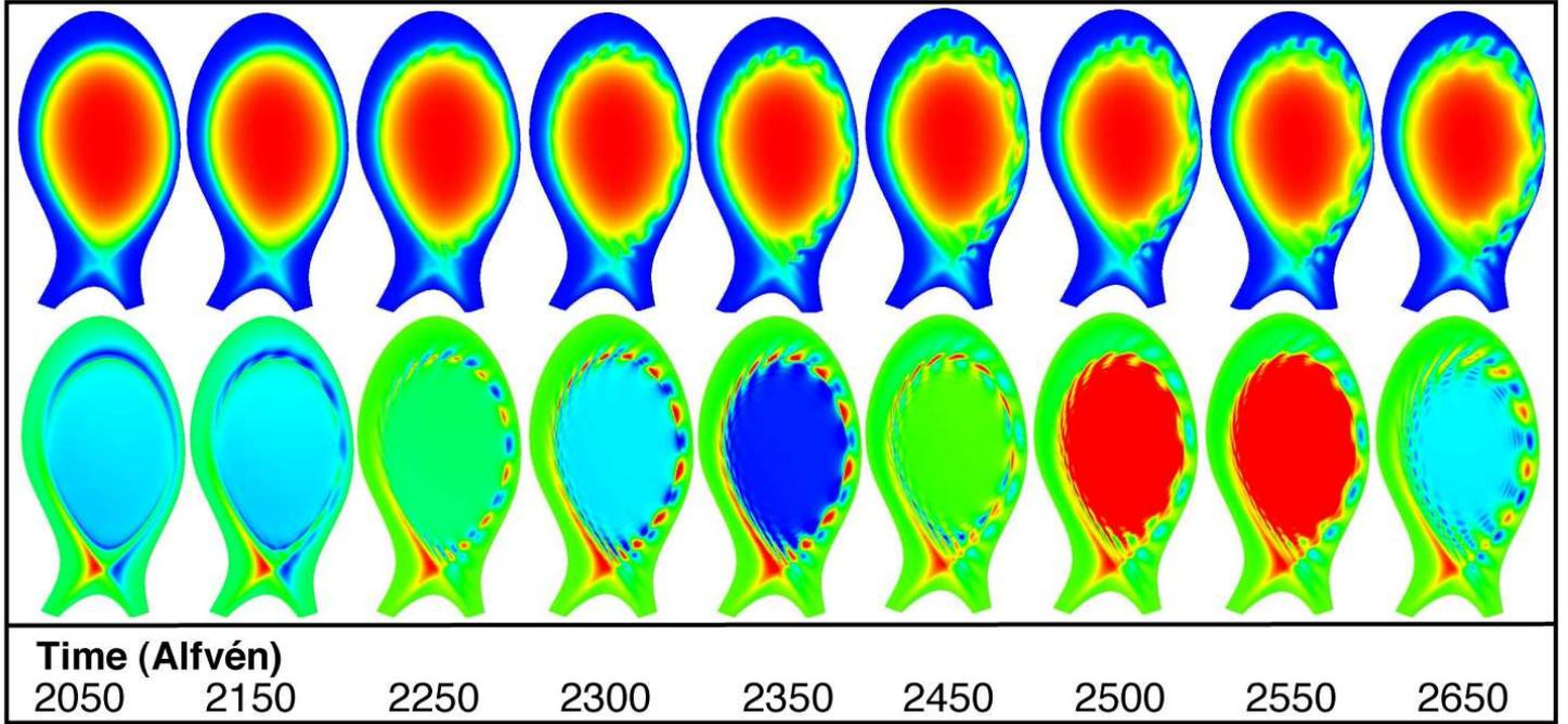
**FIGURE 1.** Non-linear Simulation of a Ballooning Mode (ELM). Top row shows the density filaments coming through the separatrix, and bottom row shows the electric potential with strong  $m = 0$  structure.
